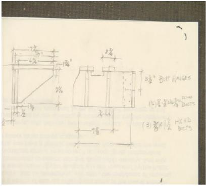
then glued the ply pieces together. The curved shape of the front of the fixture was taken from a template I created by drawing the shape of the bed end on paper.
