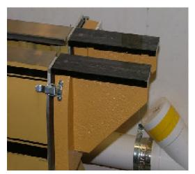
them. It's a welcome change from lifting it off and on when turning from the end of the lathe and keeps me from having to find a place to put the darn thing every time. My next project will be to secure it in some open position so that I won't have to worry about it swinging closed at the wrong time. The aluminum plate was \$12, the hinges were \$12, the bolts and screws were \$6 and the paint about \$4. Making the total cost was less than \$35.
